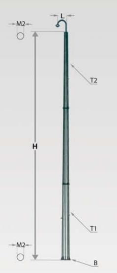
With the development of technology and increasing the areas of urban and interurban roads, the need to record events and send the information to the traffic control centers has become highly important. In order to have an appropriate view, cameras should be installed at an appropriate angle and level. In order to meet this essential need, the design and production of tubular and multihedral poles and related long arms are underway.
