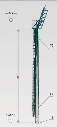
These types of towers are designed to provide appropriate and uniform lighting for sports fields for players and spectators whose height and exposure are calculated and determined based on the type of use and area of the stadium as well as the number of spectators. The basket of these towers can be fixed and movable. In a moving type, the basket is transferred by the electric motor to the bottom of the tower and the switching of the lamps and its maintenance and service is easily carries out.
